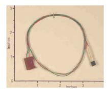
immune to noise or loading and it is ideally suited for remote sensing applications. This sensor is factory calibrated by Dallas Semi and has excellent log-time stability. In addition, this sensor has a small thermal-mass and a small OD.
